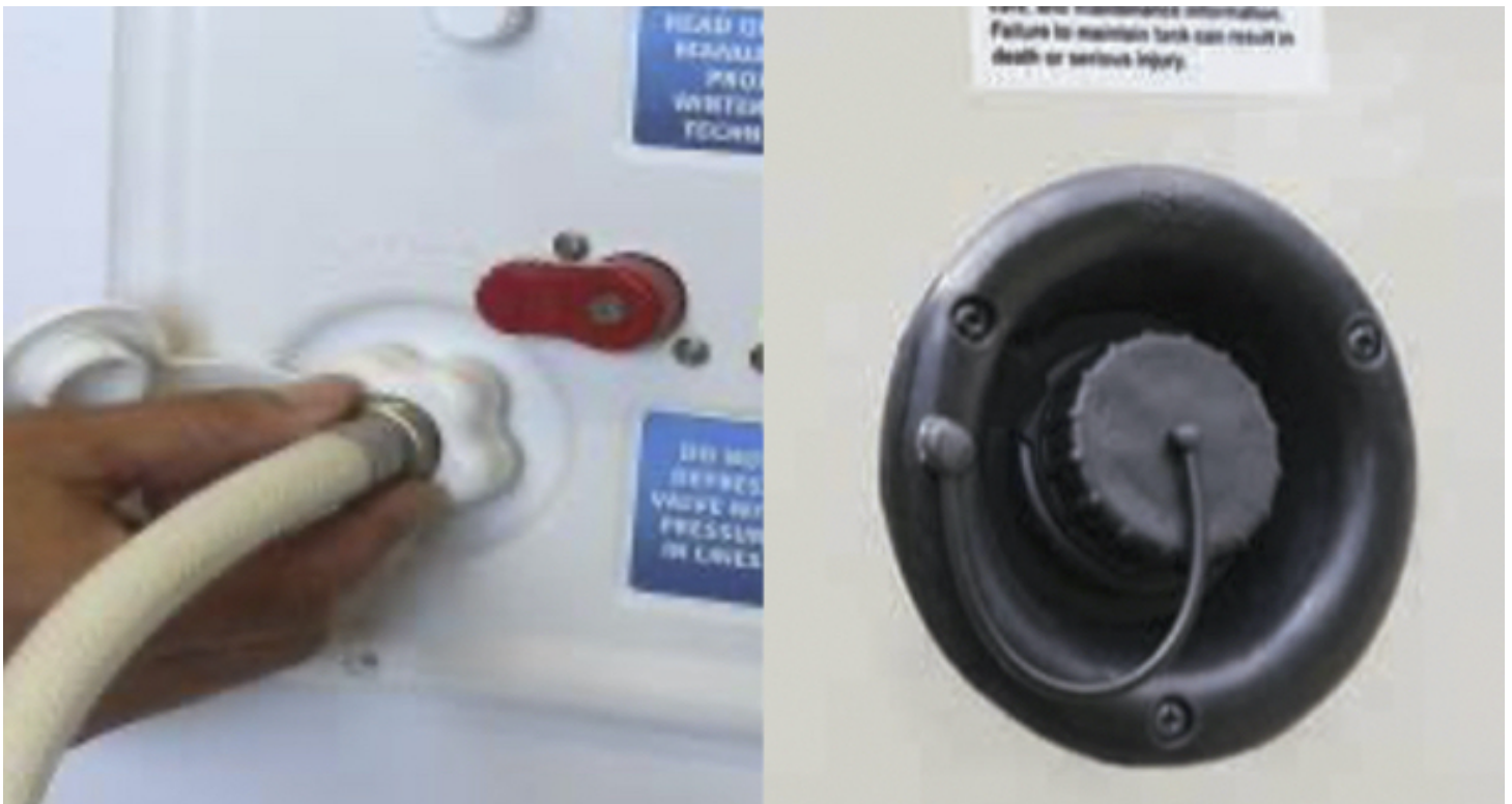
(L) Fresh water fill connection. (R) Gravity-controlled water intake.
